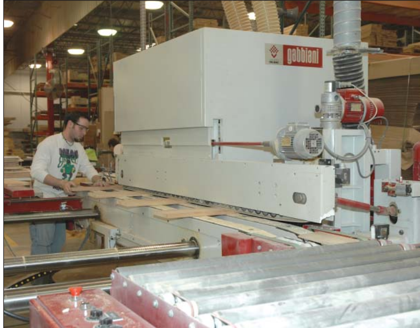
There are three Gabbiani panel lines between the two plants, two at the cabinetry plant and a new machine with barcode scanning and a return feed conveyor at the passage door plant.
