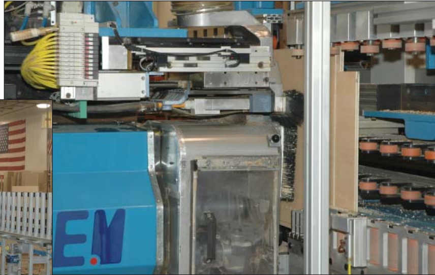
The RE.M CNC machining center, above, handles parts using a head that travels vertically with parts being secured with a roller system.
