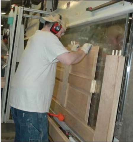
Door parts are assembled and clamped on the Systematix door press, directly across from the intricate door parts automated system.
