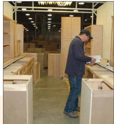
Cabinets are set up as they will be installed in a kitchen to visually check that everything matches. Even with standards, there are variations and the company checks everything before it leaves the building.
