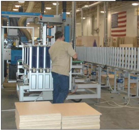
The RE.M CNC machining center, above, handles parts using a head that travels vertically with parts being secured with a roller system.
