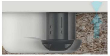
In assembly, the PEANUT head rides over the lip of the PEANUT slot and slides to the end, this action creates a strong clamping force, pulling the two panels together from the inside.
