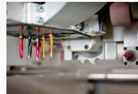
Vertical drilling unit, long edge drilling unit and grooving station
