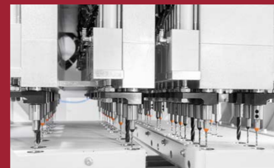
Special drilling head for vertical drilling
