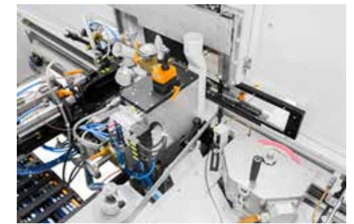
ENDMASTER-P base.line Chamfering, drilling, gluing and dowel insertion station
