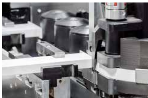
ENDMASTER K select.line edge-banding station
