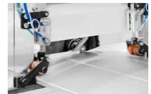
ENDMASTER-K select.line chamfering station with sensing roller
