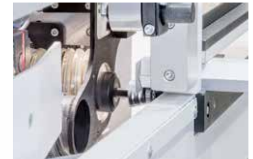
ENDMASTER-K pro.line edge-trimming station
