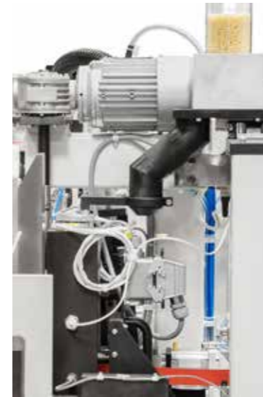
ENDMASTER-K pro.line Semi-automatic filling unit for glue granulate
