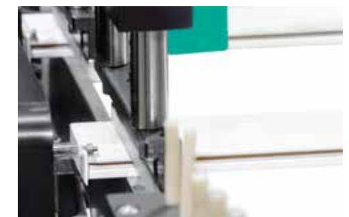
ENDMASTER-K select.line edge trimming station
