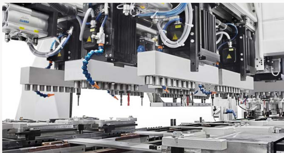
BD-B-Double-cycle Double-cycle drilling stations for two-piece processing
