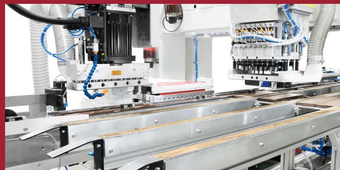
Hybrid machine featuring a combination of stationary and flexible (PTP) drilling heads
