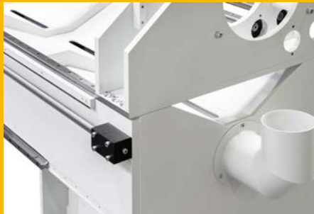
Machine bed with integrated chip-collecting system
