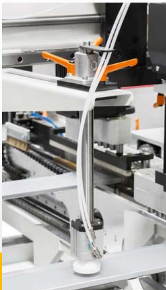
Clamping cylinder (Quick-change system at the overhead beam)
